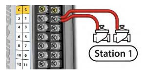
**Each screw** terminal **block** is mapped to a **single station**, meaning there are two stations mapped to each row. Multiple valves can be wired to a single station.
