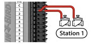
**Each row** of slots was mapped to a **single station**. Multiple valves could be wired to a single station.
