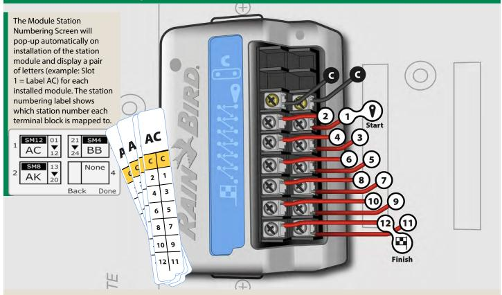
The actual station numbers will vary based on your module configuration, the example shown here is a 12 station module in Slot 1.
